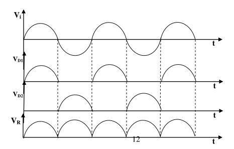
$V_{D1}$  and  $V_{D2}$  is output pd due to conduction of diode  $D_1$  and  $D_2$  respectively.
