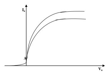
For Va = 0, electrons are emitted by the cathode with a range of speeds. A few of the electrons are emitted with sufficient kinetic energy to be able to reach the anode. This leads to a small current. If the anode is made negative relative to the cathode, a reverse current exists for negative potentials up to about 0.5V and then decreases to zero.
