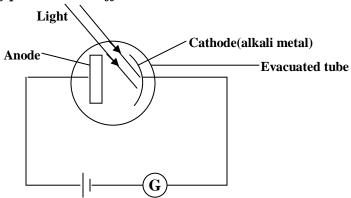
When light falls on a metal cathode, a galvanometer shows a deflection, indicating flow of current. However when the plates are covered, more current flows. Energy of the incident light is absorbed by the electrons and instantly an electron jumps out. Such ejected electrons are called photoelectrons.
