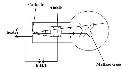
If an opaque object (Maltese cross) is placed in the path of the cathode rays, a sharp shadow of the Maltese cross is cast on the screen.
