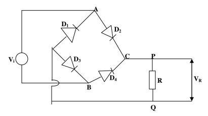
During the half cycles when A is at positive potential relative to B, diodes  $D_2$  and  $D_3$  are forward biased hence they conduct and current flows through the resistor R in the direction P to Q. Diodes  $D_1$  and  $D_4$  are reverse biased and they do not conduct. During the half cycles when B is at positive potential relative to A, diodes  $D_1$  and  $D_4$  are forward biased and they conduct. Currents flows through resistor R in the direction P to
