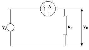
During the half cycles when A is positive relative to C the diode conducts and a p.d  $V_R$  appears across the load  $R_L$ . During the half cycles when A is at a negative potential relative to C, the diode does not conduct and no p.d appears across  $R_L$ . The a.c is half-wave rectified.
