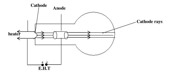
The electrons are produced at the cathode by thermionic emission and are accelerated towards the screen by the anode which is connected to the terminal of the extra high tension battery. The thermionic emission is the process whereby metal surfaces emit electrons when heated.
