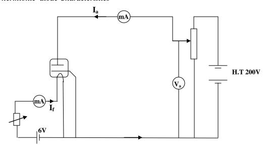
Keeping the filament current If constant, the p.d  $V_a$  between the cathode and the anode is varied. The corresponding anode current  $I_a$  is measured. A graph of  $I_a$  against  $V_a$  constitutes the anode – current anode voltage characteristics. By setting the filament current to other constant values, the corresponding  $I_a$ - $V_a$  characteristics can be obtained. These features can be shown below
