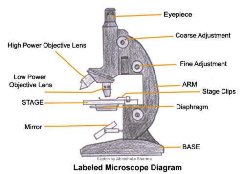
Parts of a microscope
