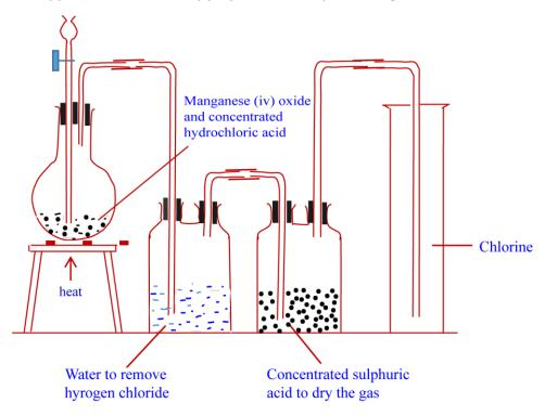
Note that chlorine is collected by downward delivery or upward displacement of air because it is denser than air
